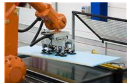
Figure 2: ABB robots handling furniture panels for Svedplan.
